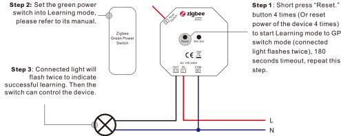
Note: Each device can learn to max. 20 zigbee green power switches.
