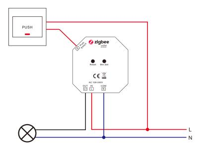
2) With Multiple Push Switches for Multiple Control Points
