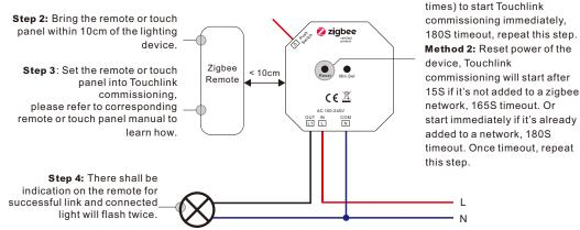
Note: 1) Directly TouchLink (both not added to a ZigBee network), each device can link with 1 remote. 2) TouchLink after both added to a ZigBee network, each device can link with max. 30 remotes. 3) To control by gateway & remote, add remote and device to network first then TouchLink. 4) After TouchLink, the device can be controlled by the linked remotes.
